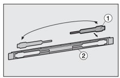
Remove cover ① from panel ②, rotate it by 180° and refit it on the other side.
